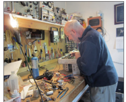
The CM-11’s CSR-5 receiver undergoing surgery by VE1FA. Numerous defective “organs” can be seen on the bench to the left of the “patient”; and yes, that propane torch was used a few times on seized hardware!
